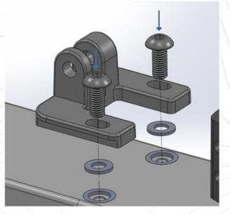
Place 1mm thick washers under the bottle bracket as shown
