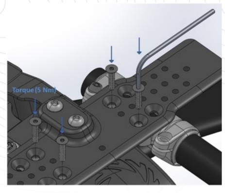
Torque the aero extension holder bolts to 5 Nm
