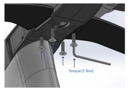
Torque the base bar bolts to 7 Nm
