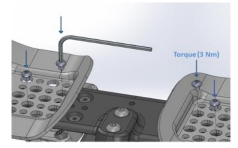
• Torque the arm cup bolts to 3 Nm
