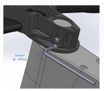
Torque the stem bolts to 6 N.m.. If necessary, they can be torqued up to 8 Nm
