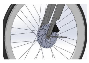
Install the thru axles and torque to 10 Nm
