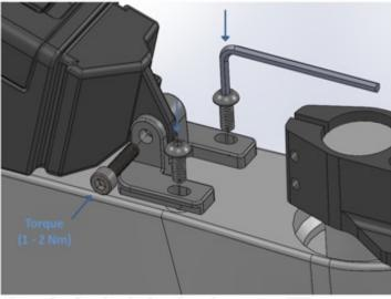
Torque the bottle bracket screws to 1 or 2 Nm
