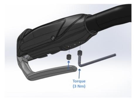
Torque the brake lever bolts to 3 Nm
