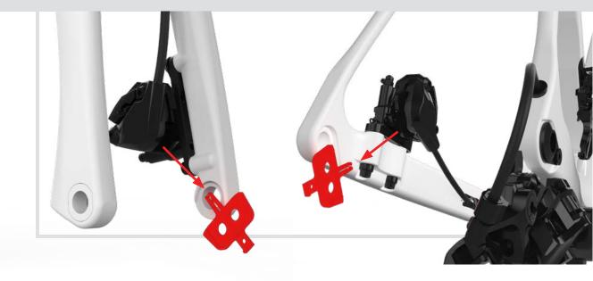
Install the wheels ensuring the rotor lines up between the brake pads
