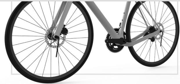
Your Ventum GS1 comes equipped with our Dual-Offset Fork. This fork has a 2-position front dropout that allows the rider to adjust the fork offset (effective steering geometry) to fine-tune their ride characteristics. The 2-position system comes with 5mm of fork offset adjustment.
